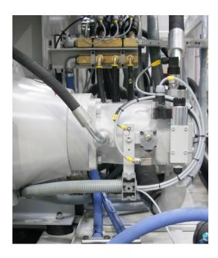
3. A frequency controlled drive system on the main motor.
