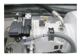
To guarantee optimal results, Stork always combines option three with option two. The pump drive system is then also modified to have pilot oil directly from the accumulators. This ensures optimal response times from the pump system. When running the machine in "eco-mode" even great energy savings are possible.
